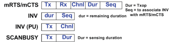
Fig. 3: Packet formats (common fields are not shown like CRC).
